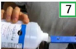
Pour Alcohol into Coupling. Repeatedly Tilt & Rotate BTL So All Coupling Inner Surfaces Are Soaked. Wait 7 minutes Then Forcibly Rotate Coupling.
