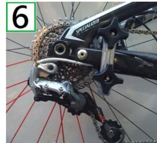
Right Side Installation Using a Clamp Accessory on Chain-Stay
