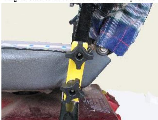
Most Secure. BTL Bolted Thru Rest Support Drill (2) ¼ in. Dia. Holes 2.6 in. apart to match Outer Clamp
