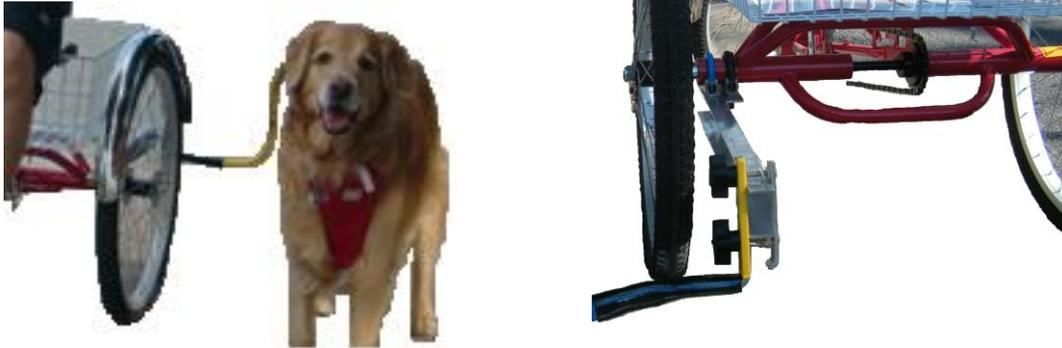
Locate adapter below axle for small dogs as in right photo above. **Locate adapter close to wheel above axle, as photo on left, for medium to large dogs. If fender mount or brakes interfere with above axle location place adapter below axle as in photo below.** Use a ½ inch wrench to tighten clamps securely so adapter will not rotate. If there is interference with clamping above or below axle go to alternate position and adjust the mast accordingly for dog's height.
